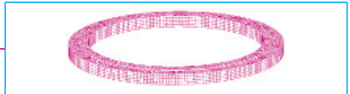
Finite elements model of the slewing bearing
